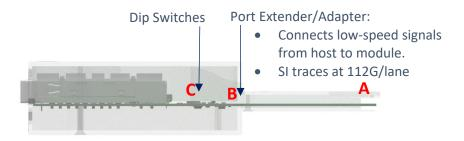
A: Signals from host side at NX-HW plug
